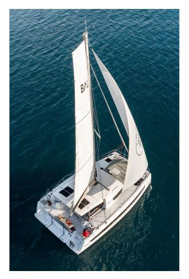
S P E C I F I C A T I O N S Length (LOA) 12.84 metres Beam 7.07 metres Displacement 11.4 tonnes Draft 1.22 metres Range 400 nautical miles under engine Engines 2 x 29 to 47,5 hp\*, Sail drive Number of cabins Owner's Version 3 Classification CE Category: Cat. A 10 persons Base price (Ex taxes/Owners Version) €345,000.00
